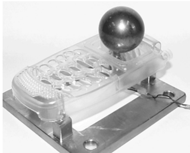
Accelerometer mounted bottom-side of lens
